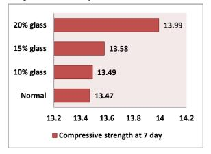
Determination of compressive strength at 7 day after curing
