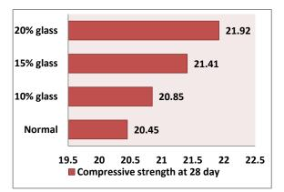
Determination of compressive strength at 28 day after curing
